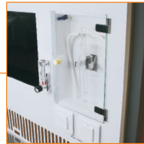
Built-in system for premixed gas supply and humidification
